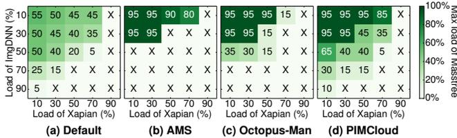
**Fig. 8: Colocation of Xapian, ImgDNN and Masstree.** Each cell represents the max RPS (as a percentage of *max load*) of Masstree when Xapian and ImgDNN run at given RPS (x and y axes), and all three applications meet QoS. Crossmarks mean that QoS cannot be met concurrently.
