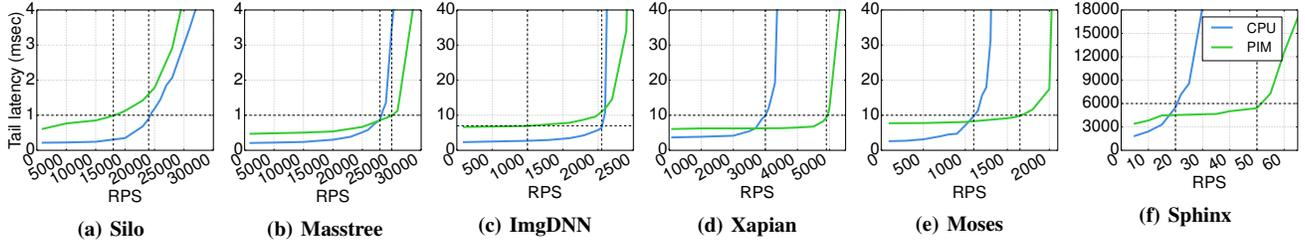
Fig. 2: Tail latency with increasing input load (RPS) on the main CPU and PIM stacks. Horizontal lines show the knee of the CPU curve, which defines QoS. Vertical lines show *max load* (maximum RPS under QoS) achieved on the main CPU and PIM stacks.
